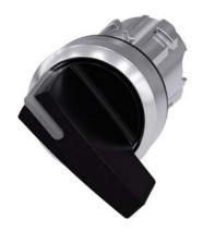
Illuminable selector switch, 22 mm, round, metal shiny, black, Selector switch long, 2 switch positions O<I, momentary contact type, Actuating angle 45°, 10:30/12, Z=50-unit packaging
