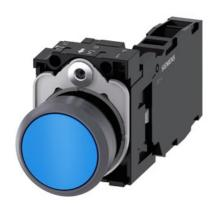
Pushbutton, 22 mm, round, plastic with metal front ring, blue, pushbutton, flat, momentary contact type, with holder, 1 NO+1 NC, screw terminal, Z=20-unit packaging
