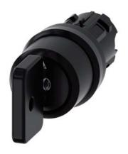
Key-operated switch O.M.R, 22 mm, round, plastic, lock number 73034, black, with 2 keys, 3 switch positions I>O<II, momentary contact type, actuating angle 2x45°, 10:30h/12h/13:30h, key removal O, with laser labeling, upper case
