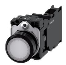
Illuminated pushbutton, 22 mm, round, plastic, white, pushbutton, flat, momentary contact type, with holder, 1 NO+1 NC, LED module with integrated LED 110 V AC, spring-type terminal, with laser labeling, upper case and lower case, always upper case at beginning of line
