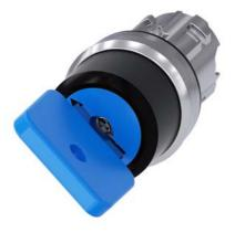
Key-operated switch O.M.R, 22 mm, round, metal, shiny, lock number 73038, blue, with 2 keys, 2 switch positions O-I, latching, actuating angle 90°, 10:30h/13:30h, key removal O, with laser labeling, upper case and lower case, always upper case at the beginning of the word
