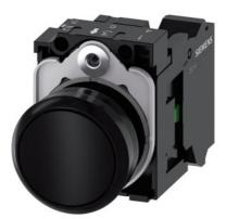
Pushbutton, 22 mm, round, plastic, black, pushbutton, flat, momentary contact type, with holder 1 NO, spring-type terminal, with laser labeling, lower case
