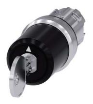
Key-operated switch BKS, 22 mm, round, metal, shiny, lock number S1, with 2 keys, 3 switch positions I-O<II, left latching, right momentary contact type, actuating angle 2x45°, 10:30h/12h/13:30h, key removal O+I, with laser labeling, upper case and lower case, always upper case at beginning of line
