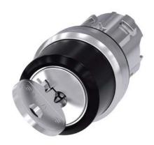
RONIS key-operated switch, 22 mm, round, metal, shiny, lock number 455, with 2 keys, 2 switch positions O<I, momentary contact type, Actuating angle 45°, 10:30h/12h, key removal O, with laser labeling, lower case
