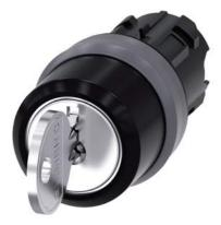
RONIS key-operated switch, 22 mm, round, plastic with metal front ring, special lock, with 2 keys, 3 switch positions I-O<II, left latching, right momentary contact type, actuating angle 2x45°, 10:30h/12h/13:30h, key removal I, possible special locks: SB31, 421, 455
