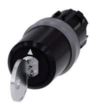
key-operated switch Siemens, 22 mm, round, plastic with metal front ring, lock number SSG10, with 2 keys, 3 switch positions I>O<II, momentary contact type, actuating angle  $2x45^{\circ}$ , 10:30h/12h/13:30h, key removal O, with laser labeling, upper case
