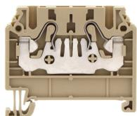
Feed-through terminal, Push-in connection, Mounting type: Mounting rail TS 35/7.5, Rated cross-section: 1.5 mm<sup>2</sup>, Width: 4.1 mm, Colour: Beige
