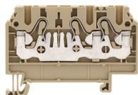
Feed-through terminal, Push-in connection, Mounting type: Mounting rail TS 35/7.5, Rated cross-section: 1.5 mm<sup>2</sup>, Width: 4.1 mm, Colour: Beige
