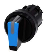
Selector switch, illuminable, 22 mm, round, plastic, blue, selector switch, short, 3 switch positions I-O-II, latching, actuating angle 2x45°, 10:30h/12h/13:30h, with laser labeling, inscription or symbol Customerspecific selection with SIRIUS ACT configurator (CIN)
