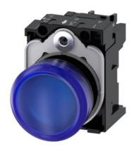
Indicator lights, 22 mm, round, plastic, blue, lens, smooth, with holder, LED module, with integrated LED 230 V AC, screw terminal, with laser labeling, inscription or symbol Customer-specific selection with SIRIUS ACT configurator (CIN)
