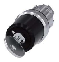
Key-operated switch BKS, 22 mm, round, metal, shiny, Lock number E1 (VW), without key, 2 switch positions O-I, latching, actuating angle 90°, 10:30h/13:30h, key removal O+I, with laser labeling, upper case and lower case, always upper case at beginning of line
