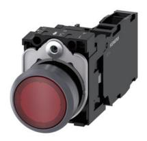
Illuminated pushbutton, 22 mm, round, plastic with metal front ring, red, pushbutton, flat, momentary contact type, with holder, 1 NO+1 NC, LED module with integrated LED 110 V AC, screw terminal, with laser labeling, upper case
