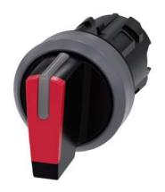
Selector switch, illuminable, 22 mm, round, plastic with metal front ring, red, selector switch, short, 3 switch positions I>O<II, momentary contact type, actuating angle  $2x45^{\circ}$ , 10:30h/12h/13:30h, with laser labeling, upper case
