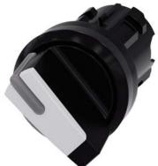
Selector switch, illuminable, 22 mm, round, plastic, white, selector switch, short, 2 switch positions O<I, momentary contact type, Actuating angle 45°, 10:30h/12h, with laser labeling, upper case and lower case, always upper case at the beginning of the word
