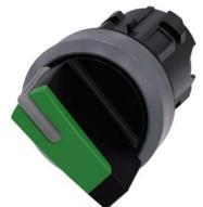
Selector switch, illuminable, 22 mm, round, plastic with metal front ring, green, selector switch, short, 2 switch positions O-I, latching, actuating angle 90°, 10:30h/13:30h, Z=50-unit packaging
