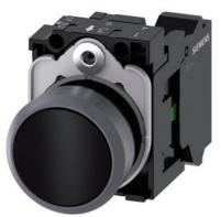
Pushbutton, 22 mm, round, plastic with metal front ring, black, pushbutton, flat, momentary contact type, with holder, 1 NO, spring-type terminal, with laser labeling, inscription or symbol Customer-specific selection with SIRIUS ACT configurator (CIN)
