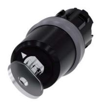
key-operated switch Siemens, 22 mm, round, plastic with metal front ring, lock no. LSG1, with 2 keys, 2 switch positions O-I, latching, actuating angle 90°, 10:30h/13:30h, key removal O+I, Z=50-unit packaging
