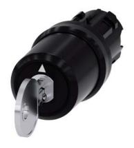
key-operated switch Siemens, 22 mm, round, plastic, lock number SSG10, with 2 keys, 3 switch positions I-O<II, left latching, momentary contact type on the right, actuating angle  $2x45^{\circ}$ , 10:30h/12h/13:30h, key removal O, with laser labeling, upper case and lower case, always upper case at the beginning of the word
