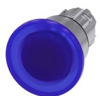
Illuminated mushroom pushbutton, 22 mm, round, metal, shiny, blue, 40 mm, latching, pull-to-unlatch mechanism, with laser labeling, upper case and lower case, always upper case at the beginning of the word
