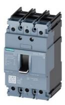
circuit breaker 3VA5 UL frame 125 breaking capacity class M 35kA @ 480 V 3-pole, line protection TM210, FTFM, In=80A overload protection Ir=80A fixed short-circuit protection Ii=10 x In UL489 SB (naval), 50 deg. cel. cable connection on both sides
