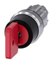
Key-operated switch O.M.R, 22 mm, round, metal, shiny, lock number 73037, red, with 2 keys, 3 switch positions I-O-II, latching, actuating angle 2x45°, 10:30h/12h/13:30h, Key removal I+O+II, with laser labeling, upper case and lower case, always upper case at beginning of line
