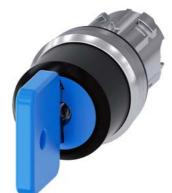
Key-operated switch O.M.R, 22 mm, round, metal, shiny, lock number 73038, blue, with 2 keys, 3 switch positions I-O-II, latching, actuating angle 2x45°, 10:30h/12h/13:30h, Key removal I+O+II, with laser labeling, inscription or symbol Customer-specific selection with SIRIUS ACT configurator (CIN)
