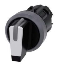
Selector switch, illuminable, 22 mm, round, plastic with metal front ring, white, selector switch, short, 3 switch positions I-O-II, latching, actuating angle  $2x45^{\circ}$ , 10:30h/12h/13:30h, Z=50-unit packaging
