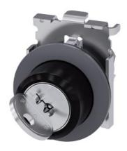
RONIS key-operated switch, 30 mm, round, Metal, matte, front ring for flush installation, lock number SB30, with 2 keys, 2 switch positions O-I, latching, actuating angle 90°, 10:30h/13:30h, key removal O+I, possible special locks: SB31, 421, 455, with laser labeling, inscription or symbol Customerspecific selection with SIRIUS ACT configurator (CIN)
