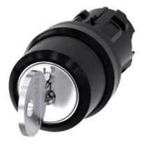
RONIS key-operated switch, 22 mm, round, plastic, lock number SB30, with 2 keys, 3 switch positions I-O-II, latching, actuating angle 2x45°, 10:30h/12h/13:30h, key removal I, possible special locks: SB31, 421, 455, with laser labeling, upper case and lower case, always upper case at the beginning of the word
