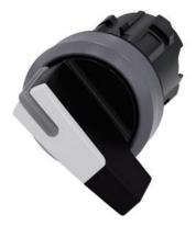
Selector switch, illuminable, 22 mm, round, plastic with metal front ring, white, selector switch, long, 2 switch positions O-I, latching, actuating angle  $90^{\circ}$ , 10:30h/13:30h, with laser labeling, upper case
