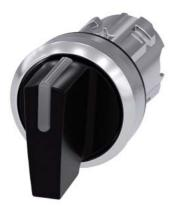
Illuminable selector switch, 22 mm, round, metal shiny, black, Selector switch short, 3 switch positions I>O<II, momentary contact on the left, latching on the right, actuating angle  $2x45^{\circ}$ , 10:30 /12 /13:30, Z=50-unit packaging
