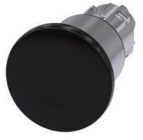
Mushroom pushbutton, 22 mm, round, metal, shiny, black, 40 mm, 3 switch positions, latches after pushing in, unlatches by pull-to-unlatch mechanism to center position, after pulling out the button Retraction to center position, with laser labeling, upper case and lower case, always upper case at the beginning of the word
