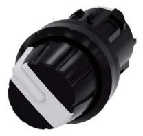
Selector switch, 22 mm, round, plastic, white, Rotary knob, 4 switch positions I-II-III-IV, latching, Actuating angle  $4x90^\circ$ , 3h/6h/9h/12h, with laser labeling, upper case
