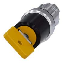
Key-operated switch O.M.R, 22 mm, round, metal, shiny, lock number 73033, yellow, with 2 keys, 2 switch positions O-I, latching, actuating angle 90°, 10:30h/13:30h, key removal O+I, with laser labeling, upper case and lower case, always upper case at the beginning of the word
