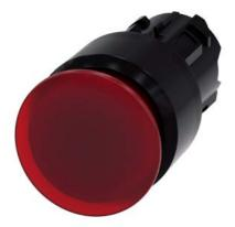
Illuminated mushroom pushbutton, 22 mm, round, plastic, red, 30 mm, latching, pull-to-unlatch mechanism, with laser labeling, upper case
