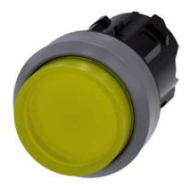
Illuminated pushbutton, 22 mm, round, plastic with metal front ring, yellow, pushbutton, raised momentary contact type, with laser labeling, symbol number according to, ISO 7000 or IEC 60417
