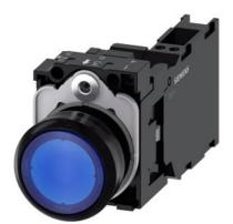
Illuminated pushbutton, 22 mm, round, plastic, blue, pushbutton, flat, momentary contact type, with holder, 1 NO+1 NC, LED module with integrated LED 110 V AC, spring-type terminal, with laser labeling, inscription or symbol Customer-specific selection with SIRIUS ACT configurator (CIN)
