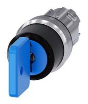
Key-operated switch O.M.R, 22 mm, round, metal, shiny, lock number 73038, blue, with 2 keys, 3 switch positions I-O-II, latching, actuating angle 2x45°, 10:30h/12h/13:30h, Key removal I+O+II, Z=50-unit packaging
