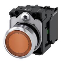
Illuminated pushbutton, 22 mm, round, metal, shiny, amber, pushbutton, flat, momentary contact type, with holder, 1NO, LED module with integrated LED 24 V AC/DC, screw terminal, with laser labeling, upper case and lower case, always upper case at beginning of line
