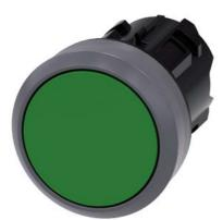
Pushbutton, 22 mm, round, plastic with metal front ring, green, pushbutton, flat, latching, Push-to-release mechanism, with laser labeling, upper case and lower case, always upper case at beginning of line
