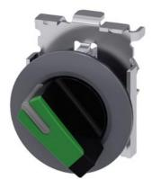
Selector switch, illuminable, 30 mm, round, Metal, matte, green, selector switch, short, front ring for flush installation, 2 switch positions O-I, latching, actuating angle  $90^{\circ}$ , 10:30h/13:30h, with laser labeling, upper case and lower case, always upper case at the beginning of the word
