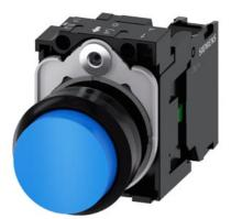
Pushbutton, 22 mm, round, plastic, blue, pushbutton, raised, momentary contact type, with holder 1 NO, screw terminal, with laser labeling, inscription or symbol Customer-specific selection with SIRIUS ACT configurator (CIN)
