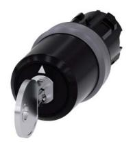
key-operated switch Siemens, 22 mm, round, plastic with metal front ring, lock number SSG10, with 2 keys, 3 switch positions I-O-II, latching, actuating angle 2x45°, 10:30h/12h/13:30h, key removal I+II, Z=50-unit packaging
