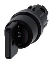
Key-operated switch O.M.R, 22 mm, round, plastic, lock number 73034, black, with 2 keys, 3 switch positions I-O-II, latching, actuating angle 2x45°, 10:30h/12h/13:30h, Key removal I+O+II Z=50-unit packaging
