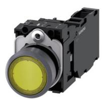
Illuminated pushbutton, 22 mm, round, plastic with metal front ring, yellow, pushbutton, flat, momentary contact type, with holder, 1 NO+1 NC, LED module with integrated LED 230 V AC, screw terminal, with laser labeling, upper case
