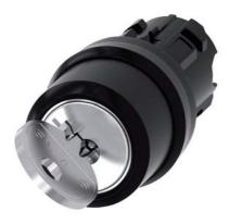
RONIS key-operated switch, 22 mm, round, plastic, Lock No. 421, with 2 keys, 2 switch positions O-I, latching, actuating angle  $90^\circ$ , 10:30h/13:30h, key removal O+I, with laser labeling, upper case and lower case, always upper case at beginning of line
