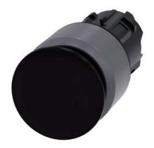
Mushroom pushbutton, 22 mm, round, plastic with metal front ring, black, 30 mm, latching, pull-to-unlatch mechanism, with laser labeling, upper case
