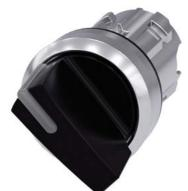
Illuminable selector switch, 22 mm, round, metal shiny, black, Selector switch short, 2 switch positions O<I, momentary contact type, Actuating angle 45°, 10:30/12, Z=50-unit packaging
