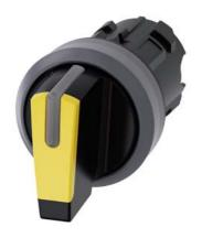
Selector switch, illuminable, 22 mm, round, plastic with metal front ring, yellow, selector switch, short, 3 switch positions I>O<II, momentary contact type, actuating angle 2x45°, 10:30h/12h/13:30h, with laser labeling, upper case
