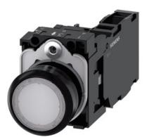
Illuminated pushbutton, 22 mm, round, plastic, white, pushbutton, flat, momentary contact type, with holder, 1 NO+1 NC, LED module with integrated LED 24 V AC/DC, screw terminal, with laser labeling, inscription or symbol Customer-specific selection with SIRIUS ACT configurator (CIN)
