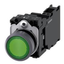
Illuminated pushbutton, 22 mm, round, plastic with metal front ring, green, pushbutton, flat, momentary contact type, with holder, 1 NO+1 NC, LED module with integrated LED 24 V AC/DC, Spring-type terminal
